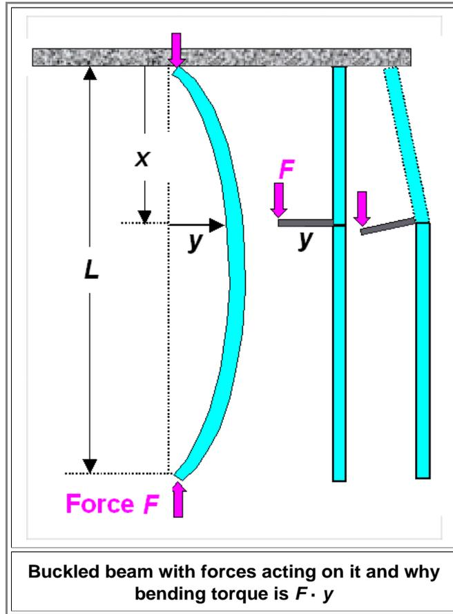
We need a force  $F$  acting on both ends with reversed signs as shown. This force induces a momentum or torque  $T(x) = F \cdot y$  if you "walk" along the buckled beam in  $x$ -direction. The drawing tries to make clear why. Using our "master" equation for beam bending, we get
