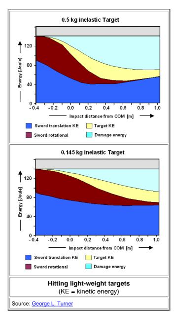
Now you deliver maximum damage energy with the tip area. In the 0,5 kg target case it is about constant for the whole tip region. However, your maximum efficiency is down to about 55 % (0,5 kg targer) or 35 % (0,145 kg target; something like a baseball). A lot of energy remains in the translational movement of the sword and also in the rotational movement. The target gets up to about 15 % of the energy just for movement, too.
