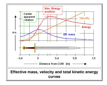
Turner doesn't supply the full set of sword data so the sword inset is from me. We can deduce the apparent center of rotation because it must be at the point where the velocity is zero.
