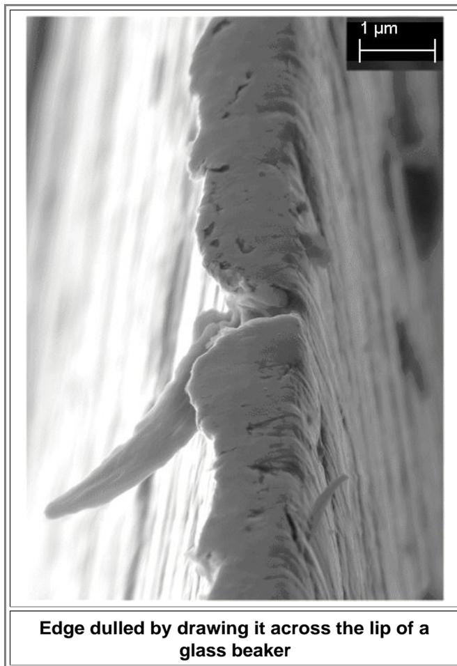
● Here we have a bit of bending but mostly deformation by compression and "filing" or abrasion, resulting in a blunt edge. Glass is just quite a bit harder than most steels and thus acts as the file; the softer steel will be the filée
