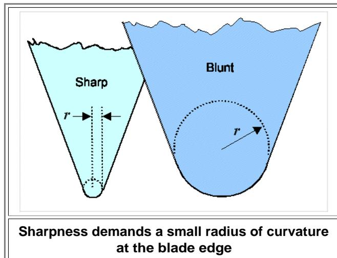
Sharpness sort of begins at a radius of curvature of a few micrometers ( $\mu\text{m}$ ). If you want "razor-sharp", you need to do better: A radius of  $0.01 \mu\text{m}$  ( $=10 \text{ nm}$ ) is a good number then. The limit, of course, is the size of an atom (imagine the circle in the picture to be an atom), giving a radius of about  $0.0001 \mu\text{m}$  or  $0.1 \text{ nm}$ . That would be a more than 10.000 fold improvement on sharpness relative to a  $1 \mu\text{m}$  radius.
