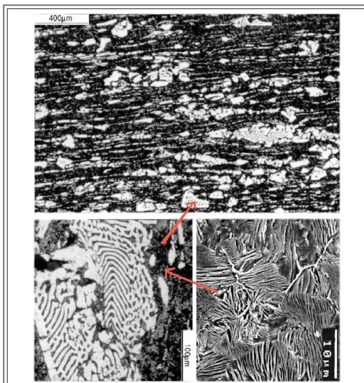
**Top: Broken up and banded cementite in a plate of tamahagane fire welded from a number of smaller pieces.**
