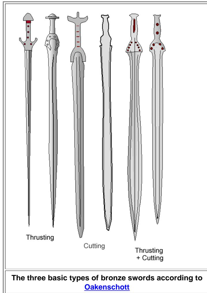
These three kinds of blades may not look all that different to you - but that is deceptive! What you can't see is that the geometry of the cross-sections is also quite different. The thrusting sword has a thick ridge running down the center, while the cutting or slashing sword is more flat (lentic-shaped) if it doesn't have outright fullers, i.e. is even thinner in the center.
