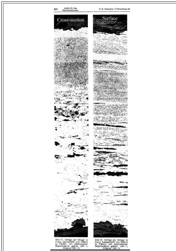
Naumann's Nital etched sections of the blade
