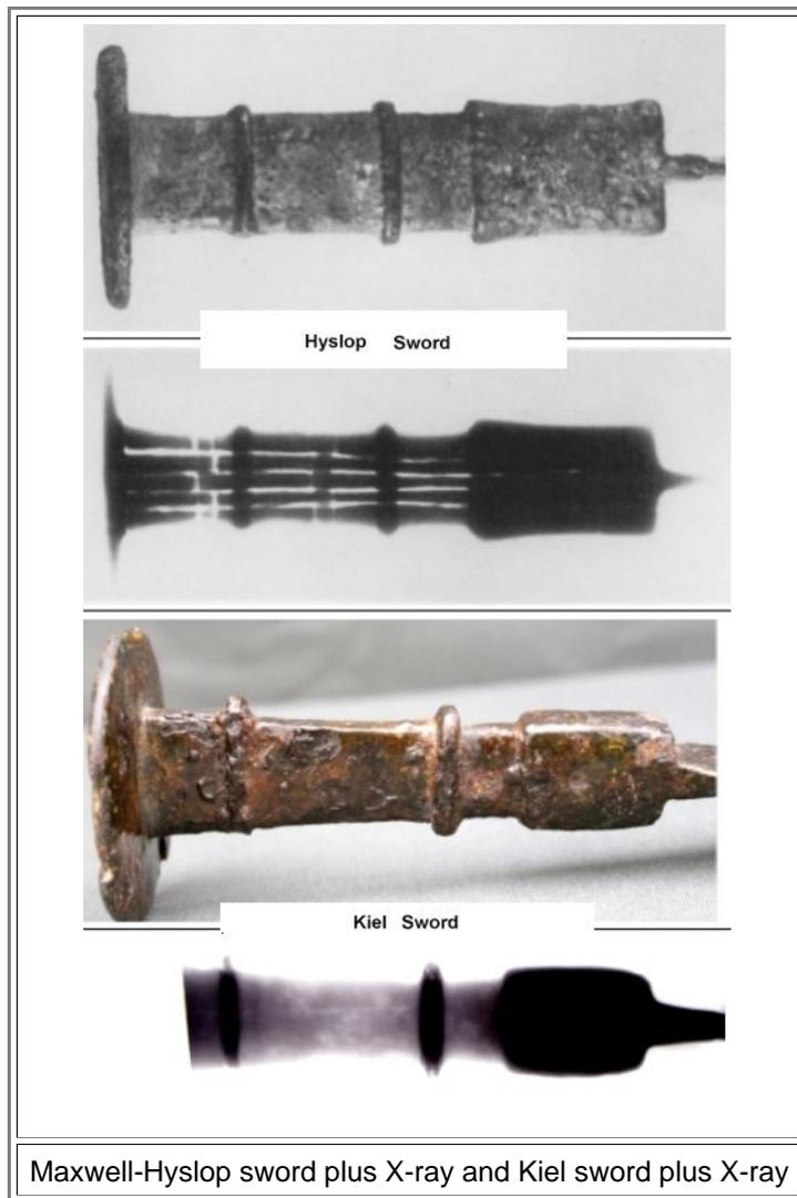
● Note that the hilt of the Hyslop sword actually consists of a stack of "thin" sheets. Fire weld the stack and you have what we found.
