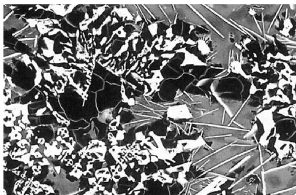
**Microstructure of some slag from copper smelting**
