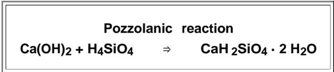
$\text{H}_4\text{SiO}_4$  is obviously a *pozzolanic* material but so are many siliceous or aluminous minerals contained in the "ashes" that volcanoes coughed up, especially in the area around the town of Pozzuoli (hence the name) west of Naples, Italy.
