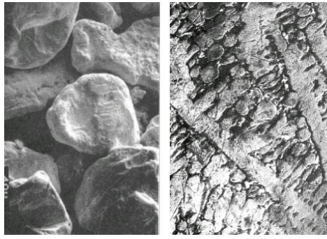
Microstructure of sintered (left) and cast (right) gold
