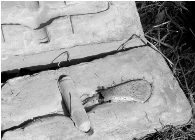
Figure 2. The partly filled mould after casting session 1
