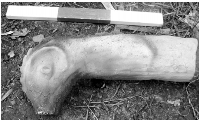
Figure 4. The partly vitrified tuyère
