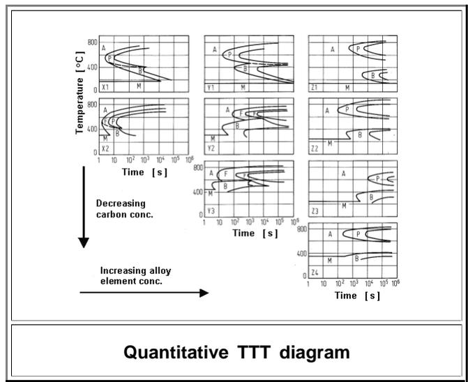
● We have steels containing the alloy elements Mn, Cr, Mo, V, Ni, W and Si in a total concentration from about 1.7 % to beyond 10 %, and carbon in concentrations from 0.2 % to 0.75 %. The (strongly simplified) TTT diagrams show not only what you will get, but also that by alloying one can indeed move the pearlite / bainite noses to the right, i.e. to larger times [as claimed above](#).
