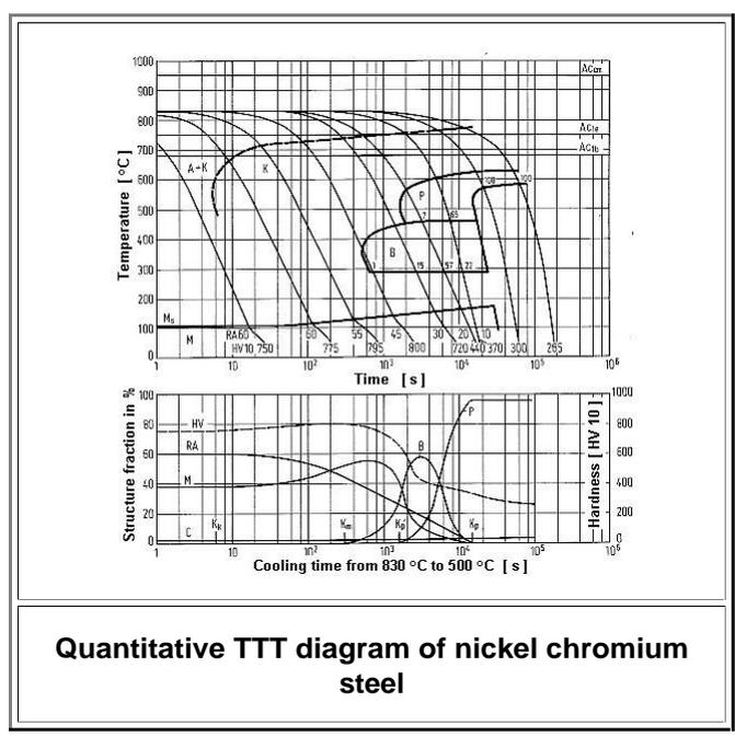
This is a quantitative TTT or better CCT diagram for a Nickel Chromium steel (14 NiCr 14) with 1.03 % carbon. In addition to the CCT diagram we have a diagram that shows how much percent of martensite (M), Bainite (B), Pearlite (P) or remaining austenite (RA) you will find, together with the Vickers hardness (HV). Note also that the "noses" appear rather late in time
