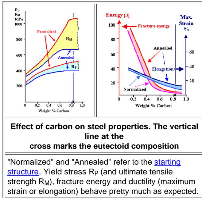
It is more or less what we expected. With increasing carbon concentration the yield strength goes up, the fracture energy down. No surprise here.
