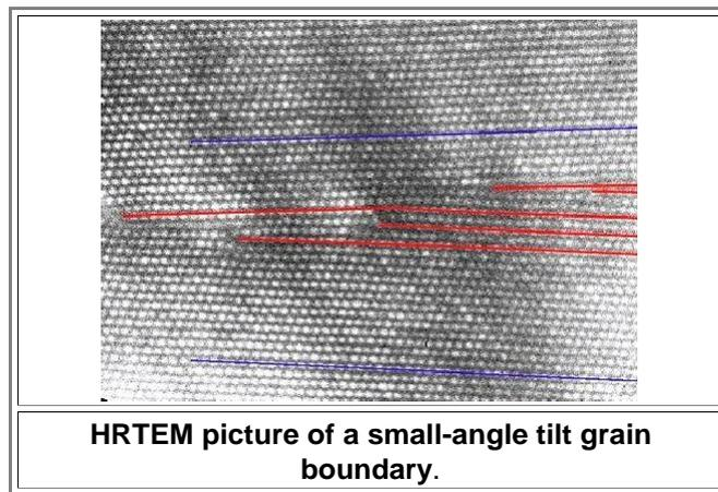
The boundary runs from left to right in the middle of the picture. The colored lines are only to guide the eye. The blue lines indicate that the orientation of the crystal above or below the boundary differs indeed by a "small angle".
