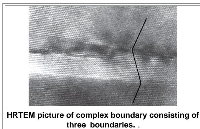
A low-angle tilt boundary composed of individual dislocations as in the picture above is actually sandwiched between two so-called "twin" boundaries, the effects of which cancel each other. That is shown by the black lines that bend substantially at the twin boundaries, but in opposite directions.
