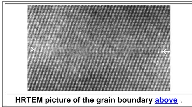
Things get a bit better with "edge-on" pictures at atomic resolution of some slightly different kind of grain boundary ("small-angle tilt").
