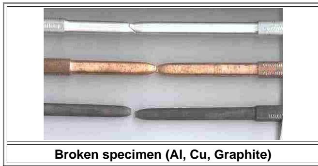
Of course, if you rip a steel paper clip apart, you need far less force than when you rip a steel sword blade apart. Since we want to get numbers for the properties of the material or **specific properties**, we want to test in such a way that the numbers we get do not depend on the specimen shape and dimensions. This requires three special measures:
