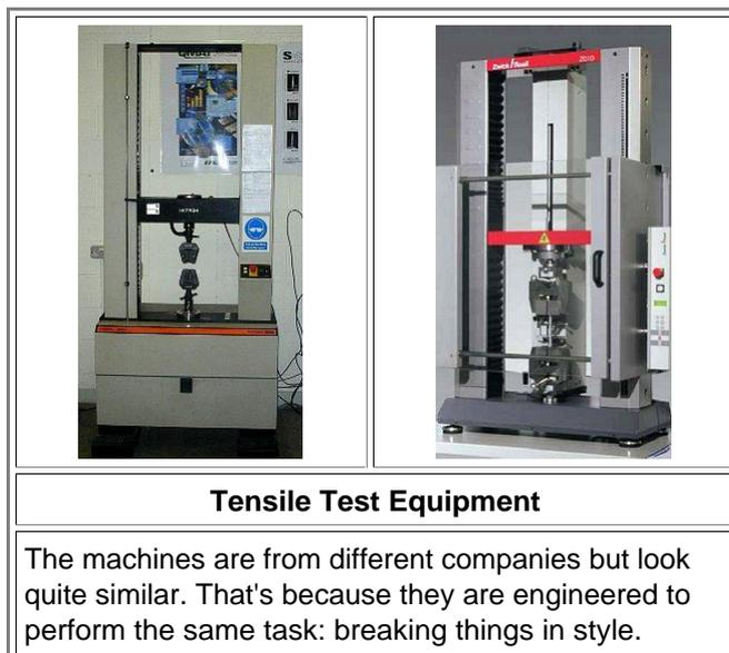
Specimen such as shown below, with standardized shape and dimensions, are clamped into the heavy jaws of the machine. The idea is to pull so that the specimen gets longer, while simultaneously recording and displaying the pulling force and the elongation.
