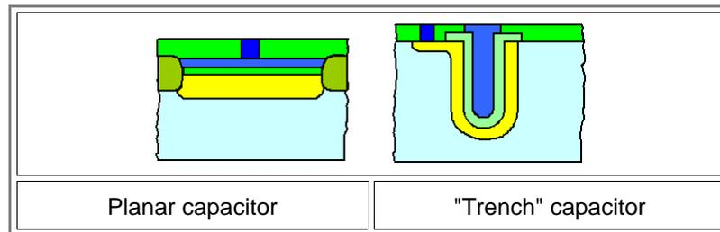
The planar capacitor (on the left) and the **"trench"** capacitor (on the right) have a doped region in the **Si** for the second electrode, which must have its own connection - in the drawing it is only shown for the trench capacitor. We learn two things from that:
