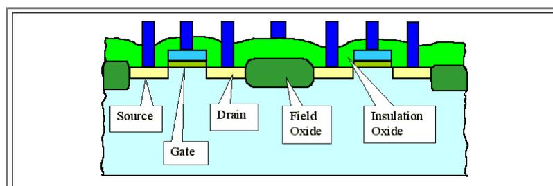
How we produce the additional insulator called **field oxide** between the transistors will concern us later; here it serves to illustrate two points:
