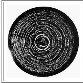
The picture was taken under "dark field" conditions. The wafer is illuminated at an angle; only light that is scattered at defects reaches the lens of the camera. Perfect areas are totally black. The defects must be due to agglomerates of the point defects (including perhaps the major impurities **O** and **C**) that were present at high temperatures - presumably in thermal equilibrium.
