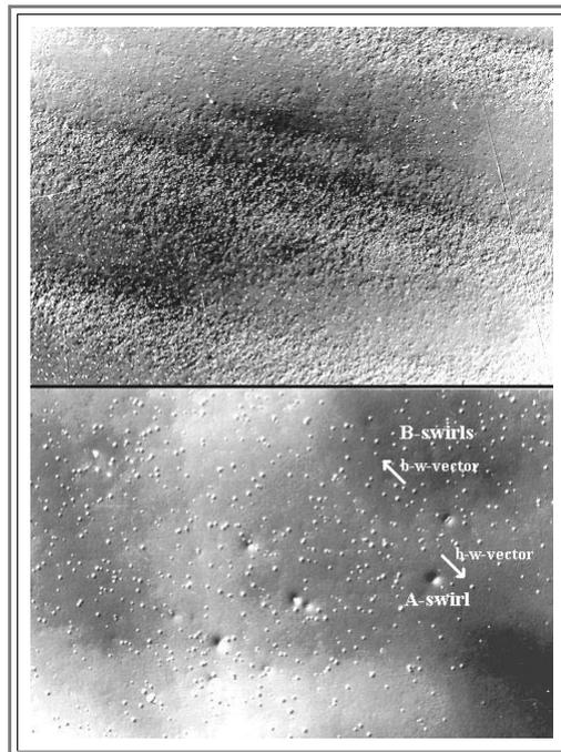
Lots of small etch pits can be seen in a striated pattern - the swirl pattern. The inner areas of the wafer may only contain these "**B-type**" defects, whereas closer to the edge of the wafer, some large hillocks - the "**A-type**" swirl defects are contained within the **B**-defects. Hillocks and pits give different signs of the black-white contrast (the vector from the black part of the contrast to the white part); this serves to distinguish between the two possibilities.
