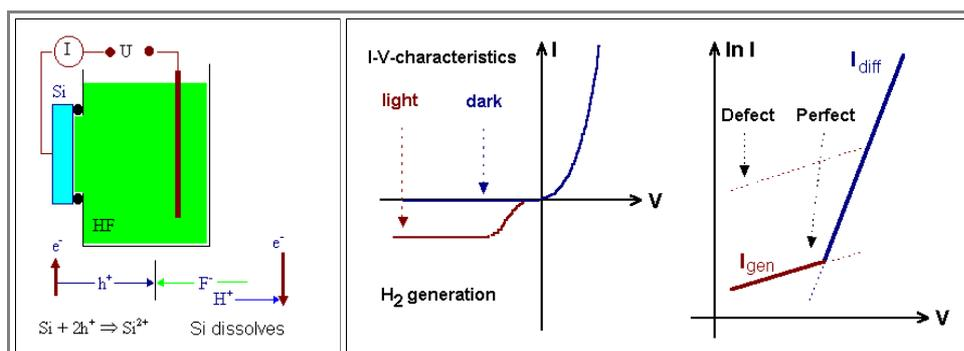
Basic experimental set-up, current flow and chemical reaction
