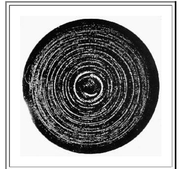
Understanding the precise nature of swirl defects was deemed to be very important for developing crystal growth techniques that could avoid these detrimental defects.
