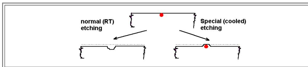
The hillocks identified the precise location of the **A-swirl** defect. A special preparation technique rendered the areas containing hillocks transparent for **TEM** investigations, and the structure of **A-swirls** defects could be identified. They consisted of dislocation loop arrangements that were generated by the agglomeration of interstitials. This gave the first direct evidence that self-interstitials are important in **Si**.
