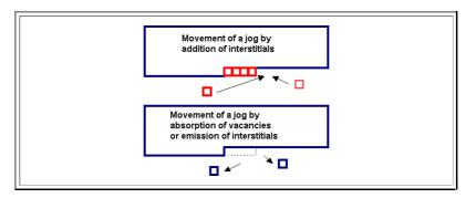
The movement of jogs by emission or absorption of point defects means that the dislocation moves. This particular process of dislocation movement is called **climb of dislocations**. It is a movement that does *not* take place in the glide plane of the dislocation.
