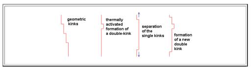
Kinks then are steps of atomic dimension in the dislocation line that are fully contained in the glide plane of the dislocation
