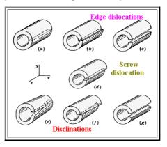
The last three cuts corresponds to special defects called disclinations that are more elementary than dislocations, but are not observed in real crystals (except, maybe, in grain boundaries). They do however, appear in two-dimensional lattices, e.g. in the flux-line lattice of a superconductor.
