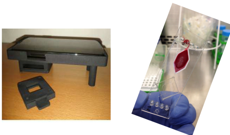
Fig. 2: (Left) Prototype for a smartphone-based optical biosensor platform. We envisage that microfluidic test chips will be inserted with the small drawer. (Right) Microfluidic chip designed with blood filter unit at the top and measurement field at the bottom.
