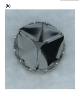
Fig. 1: First three leaflet TiNi heart valve model with 14  $\mu$ m film thickness: a) side view, b) top view.
