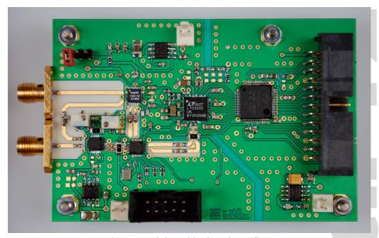
Fig. 2: Miniaturized ultra-wideband sampling oscilloscope.
