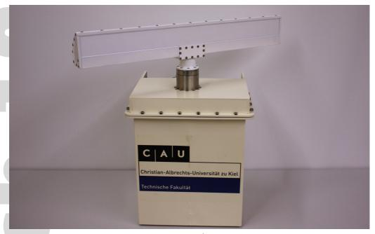
Fig. 1: Near range radar prototype.
