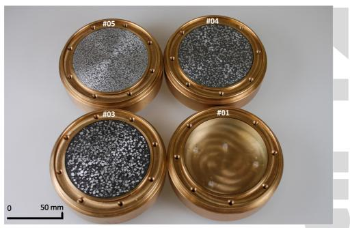
Fig. 3: Four different Cocoon-PUF prototypes fabricated with different granules/particle mass and size. Sample #01 is an ungranulated sample used for reference measurements. Samples #03, #04 and #05 are granulated samples having the same particle mass but with different randomized distribution techniques, which have been proven to have uncorrelated RF fingerprints.
