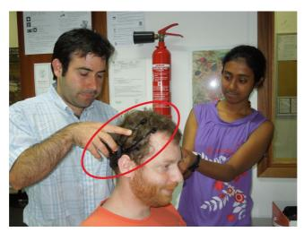
Fig. 2: Wireless EEG headset for research on brain-computer interfaces.
