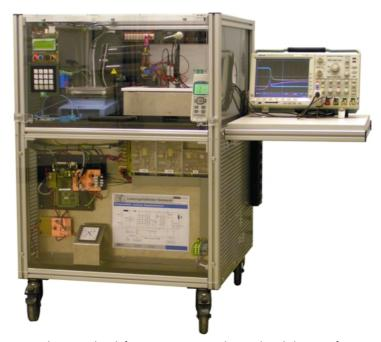
Fig. 1: New power semiconductor test bench for measurements on the switching behaviour of power semiconductors and their driver circuits up to 1200 V at different temperatures
