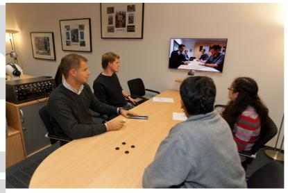
Fig. 3: Test system for multi-channel HD audio conference systems (here we use 4 compact arrays with 14 microphones in total).
