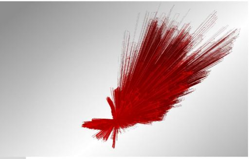
Fig. 1: Explosion. Typically, surfaces are represented through triangle meshes, where the topology (mesh connectivity) is connected with the geometry (3D points) by indexed lists. Here, the index list was corrupted, causing the very irregular geometrical structure.
