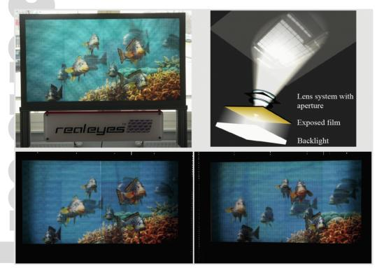
Fig. 2: Top left: Prototype of 3D Display. Top right: design of one of the 250,000 lense images on the display. Bottom: Two snapshots of the prototype 3D display showing a computer generated scene, taken from a distance of about 4.2 metres. The display shows a correct perspective for the left viewpoint (left) and the right viewpoint (right) allowing for an unconstrained 3D viewing experience.
