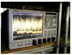
Fig. 2: Left: The four-channel 50 Gsamples/s Real-Time Oscilloscope that was utilized to realize coherent detection of optical data signals
