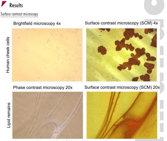
Fig. 1: Comparison of bright field, phase contrast, and surface contrast microscopy
