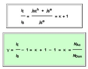
Now this is really easy! We will obtain a large current amplification (easily **100** or more), if we use a lightly doped base and a heavily doped emitter. And since we can use large base - collector voltages, we can get heavy power amplification, too.
