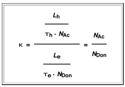
Always assuming that electrons and holes have identical lifetimes and diffusion lengths.
