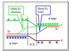
Whatever the exact positions of the Quasi-Fermi energies, their difference E<sub>F</sub>e - E<sub>F</sub>h is about equal to the difference in the bulk Fermi energy and thus
