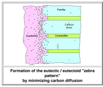
What is going on is rather clear. If the spacing of the cementite lamellae is no larger than the total diffusion lengths of the carbon atoms, all of them can get there.
