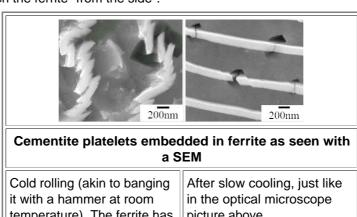
temperature). The ferrite has deformed plastically, the cementite actually fractured. picture above.
