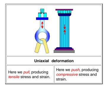
When we do a tensile test we elongate the specimen at a defined strain rate by applying the right stress via a feed-back loop.
