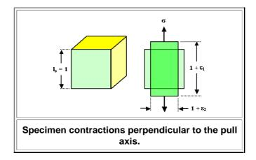
Well, we don't know so we must measure it. We have some strain ∈ 2 perpendicular to the pull direction and thus a length change of 1 + ∈2 in the geometry shown above. Since the sample gets longer but thinner, ∈2 must be negative. We have whar is called "lateral contraction".
