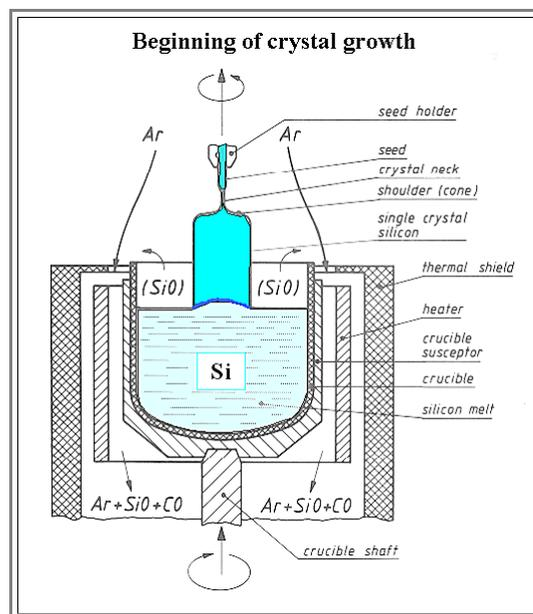
As your crystal grows, the impurity concentration (including the dopants if you do not watch out) will increase in the melt (due to [segregation](#)) and therefore also the percentage incorporated into the crystal. The temperature profile of the whole system will also change - you are now deeper down in the crucible and the crystal cools off a little more slowly. All these factors influence the homogeneity of the crystal.
