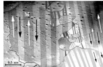
A very nice picture of the domain structure of Fe + 3% Si .
