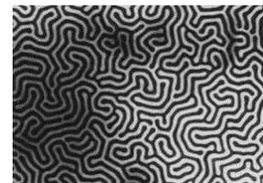
A labyrinth of magnetic domain as seen in an amorphous membrane of **Gd-Co**.
