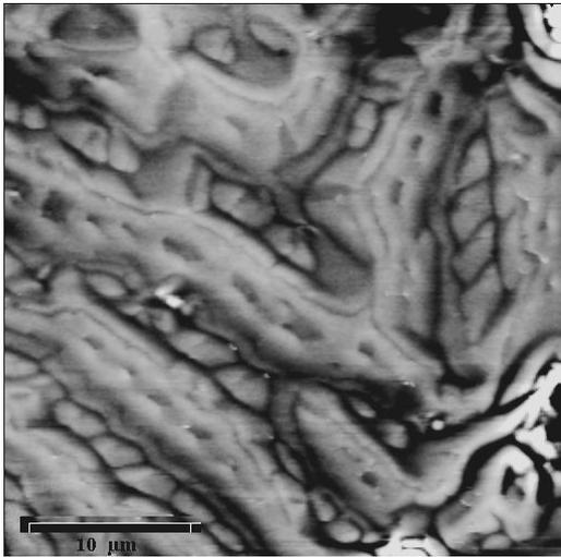
Domain structure of native *magnetite* (obtained by "magnetic force microscope imaging"). It is quite complicated.
