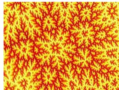
Domains in **NdFeB** material. The domain character in this highly anisotropic material depends on the orientation of the easy axis of magnetization relative to the surface. In the grain on the right the axis is oriented perpendicularly, resulting in fine branched domains, while the grain on the left has a lower degree of misorientation relative to the surface.
