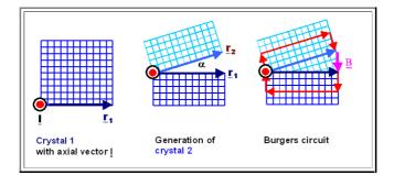
There will be a closing failure <u>B</u> which must be identical to the sum of the Burgers vectors of all the dislocations contained in the circuit. Only the *components* of the <u>b</u>'s lying in the plane perpendicular to <u>l</u> are counted, of course.
