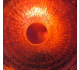
Backlit polycrystalline Si with a thickness around 5\ \mu\text{m} shows some transparency in the red.
