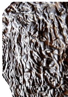
Slag from copper smelting
