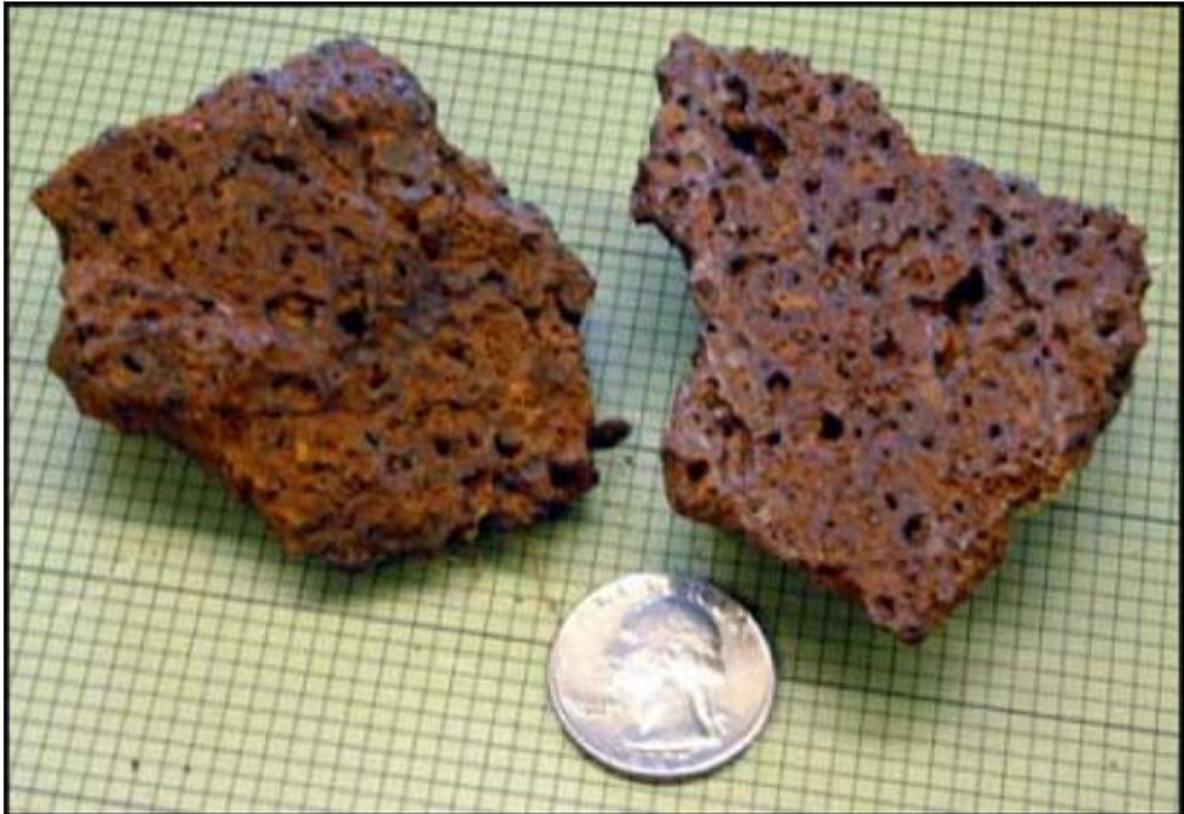
Fig. 5b Samples of "bog ore" from Nassawango Creek show vugs lined with goethite around massive "ochre".
