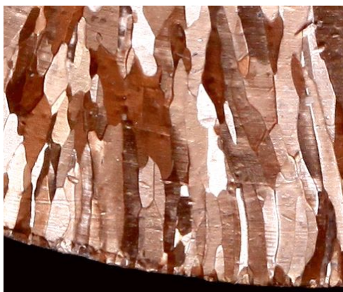
Detail of continuously cast pure copper bar (83 mm diameter)
