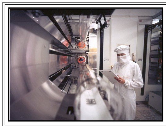
Looking along the mechanism for moving wafers into a furnace. The orange glow from the furnace tubes is visible.
