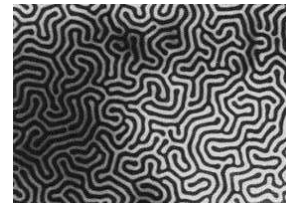
A labyrinth of magnetic domain as seen in an amorphous membrane of Gd-Co . Historical picture from unclear source.
