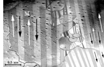
A very nice picture of the domain structure of Fe + 3% Si .
